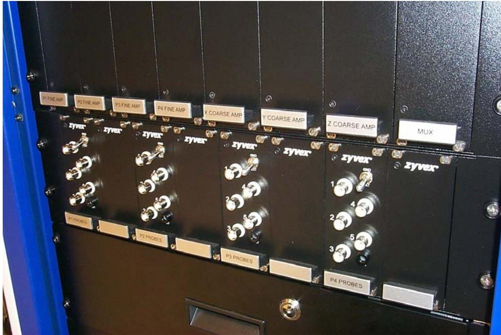
**Figure 4.4. Zyvox Patch Panel Rack**
