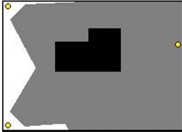
Figure 10. The yellow dots show the location of the cameras. The black boxes are occlusions, and the grey area is the effective coverage.
