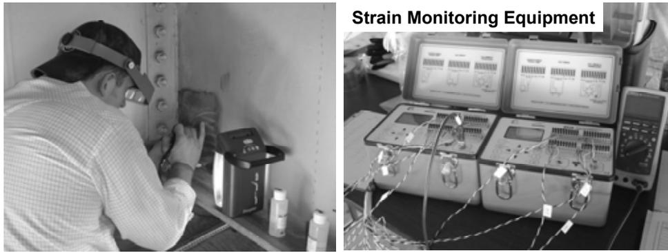
**Figure 10-13: Installation of Strain Gages in Vicinity of Fatigue Cracks**
